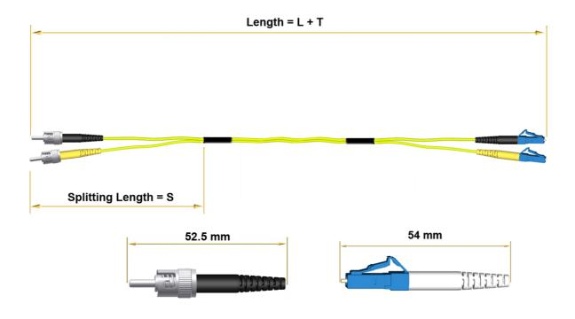
L = variable lengths T = Tolerance - 0 / + 1% L min + 10 cm
